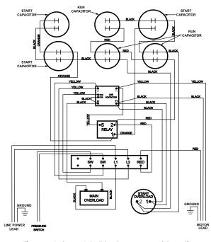
if you are not using a control switch such as a pressure switch you will need to connect a wire between the SW terminals for the panel to work.
