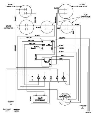
if you are not using a control switch such as a pressure switch you will need to connect a wire between the SW terminals for the panel to work.
