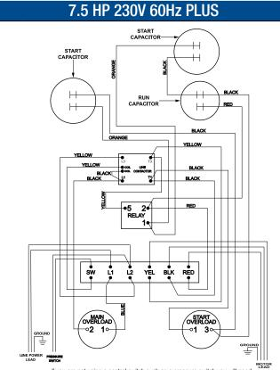
if you are not using a control switch such as a pressure switch you will need to connect a wire between the SW & L2 terminals for the panel to work.
