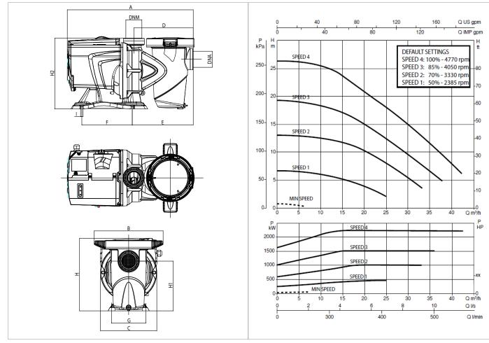
The performance curves are based on kinematic viscosity values =  $1 \text{ mm}^2$ /s and density equal to 1000 kg/m<sup>3</sup>. Curve tolerance according to ISO 9906.
