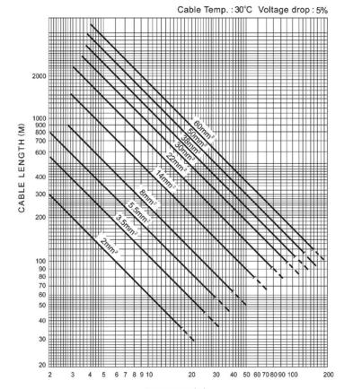
$\label{eq:current} \text{CURRENT}\left(\mathsf{A}\right) \to \\ \text{Dotted Line shows the condition of dangerous use}.$
