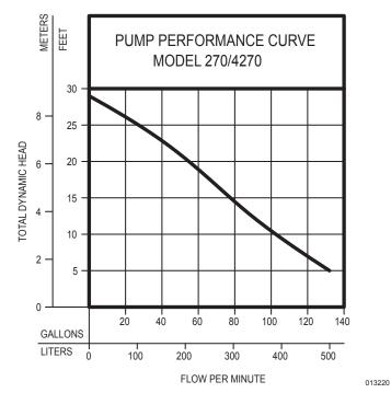
**MODEL COMPARISON** Model Seal Mode Volts Ph Amps HP Hz Lbs Kg Simplex **Duplex** BN270 115 1 15.0 1 60 49 22 Single Auto 1 or 2 3 BE270 Single Auto 230 1 7.5 1 60 73 33 1 or 2 3 N270 Single Non 115 1 15.0 1 60 49 22 1 or 2 3 73 N4270 Double Non 115 1 15.0 1 60 33 1 or 2 3 49 E270 Single Non 230 1 7.5 1 60 22 1 or 2 3 E4270 Double 1 7.5 73 33 1 or 2 3 Non 230
